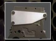
All diesel heads are resurfaced and tested for straightness and proper (Rz) surface finish to prevent head gasket failures.
