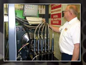
Fuel systems are calibrated with the latest computerized test equipment for precise pump adjustment.
